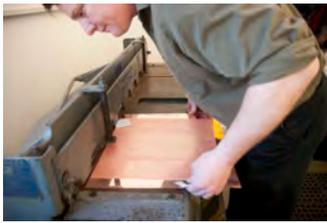
Trim the copper to the desired size. By trimming down after the etch you can take some of the pressure off placement of the image on the gel. It is a trope to leave a boarder around the image. This is only a tradition, so I tend to trim according to what the image needs visually, although boarders do seem to preserve values towards the edge of the plate.
