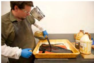
Pre mixed baths of ferric chloride are measured out in an archaic measure of specific gravity called baumé. The ferric made by Fuji Hunt works best, because it is very dense and ph neutral. Any acidity will disrupt the gel. Use two baths to keep the etch moving at the correct speed.
