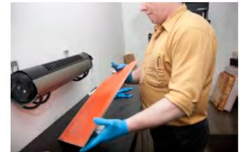
Drying the plate is the most critical step. Place in front of a low fan and rotate until there is no more dripping water. Then let the plate rest for at least 3 hours.
