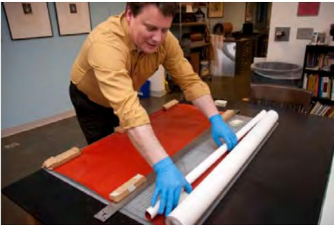
Carbon Tissue is composed of a layer of carbon tissue attached to a layer of paper. The material tends to curl based on the relative humidity of the room. Cutting the tissue will require some ingenuity to keep it flat. I use weights and rulers to keep everything in line.
