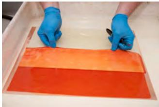
Submerge the plate in hot water and peel back the paper backing.
