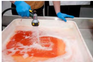
Rinse the gel to wash away all of the unexposed gel. The image will look developed before it is done. The plate is completely developed when the water rinses clean. Rinse with cold water.
