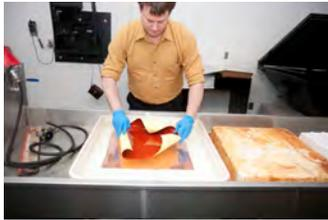
Submerge the gel in 60°F water to adhere it to the copper plate.
