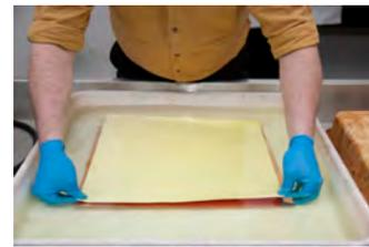
Align the gel to the plate and lift from the water avoiding air bubbles.
